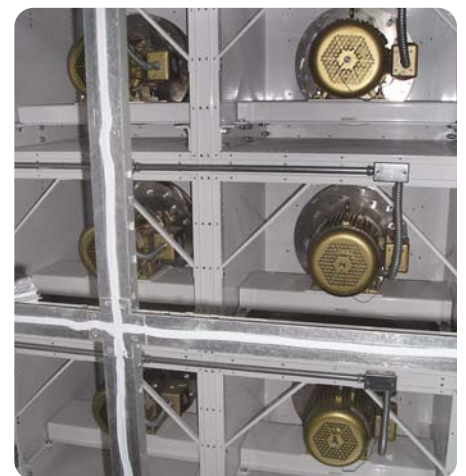
Because of its direct-drive design and smaller fan diameters, the FANWALL has a lower acoustic impact, especially in the lower frequencies, which are more difficult to attenuate.
