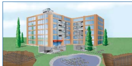
Illustration of common ground source applications where the heat sink/source is either the ground or pond.
